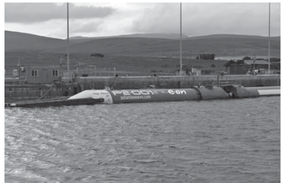
FIGURE P9.52 Pelamis P-750 wave energy converter. (Used with permission from © Doug Houghton/Alamy.)
