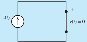
FIGURE 4.17(b) Equivalent circuit of an inductor when constant current is applied to it.
