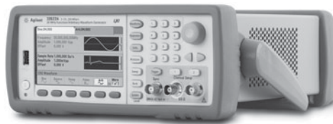
FIGURE 14.38 A function generator. (© Agilent Technologies, Inc. 2012. Reproduced with permission. Courtesy of Agilent Technologies, Inc.)
