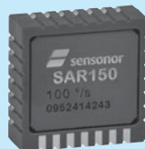
FIGURE 8.49 Circuit of a gyro sensor and photo of gyro sensor. (Photo courtesy of Sensoron Technologies AS.)
